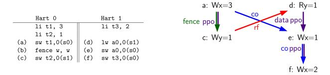
Figure A.19: Write subsumption litmus test, allowed execution.
