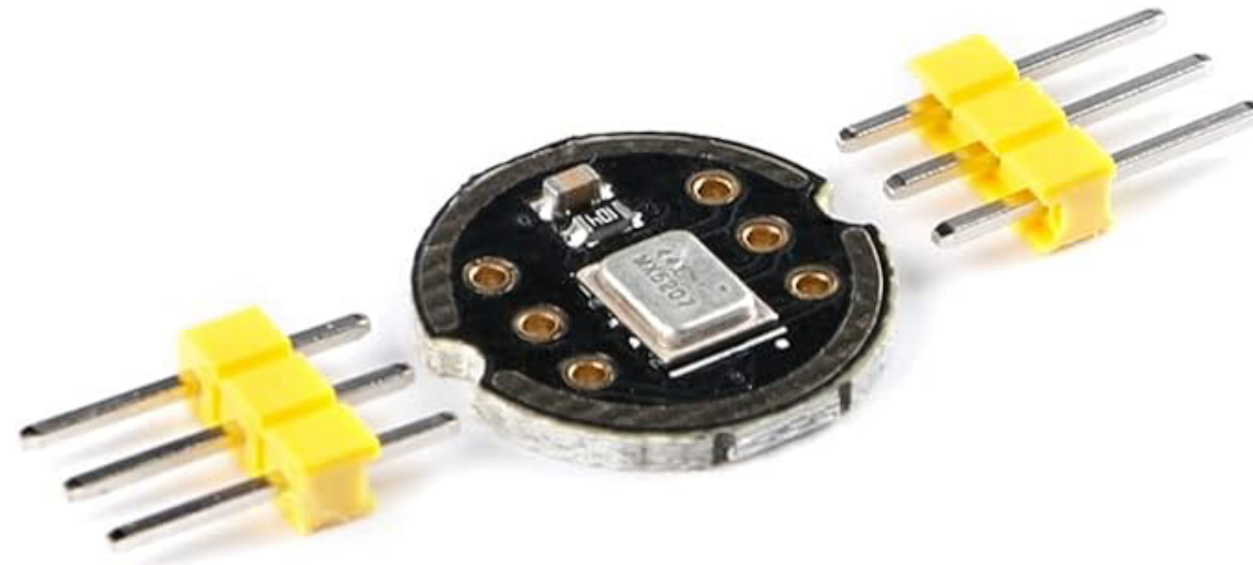
Adafruit I2S MEMS Microphone Breakout - SPH0645LM4H ( $12 on amazon.com )
