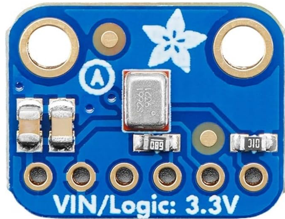
Adafruit I2S MEMS Microphone Breakout - SPH0645LM4H ( $12 on amazon.com )
